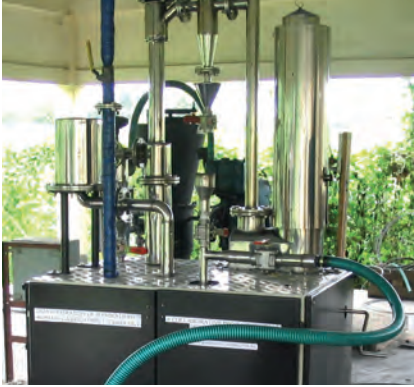
1 kW gasification based power generation system
