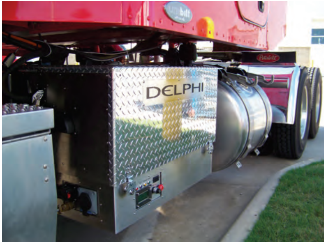
Peterbilt truck equipped with Delphi Diesel SOFC APU Technology Demonstrator
