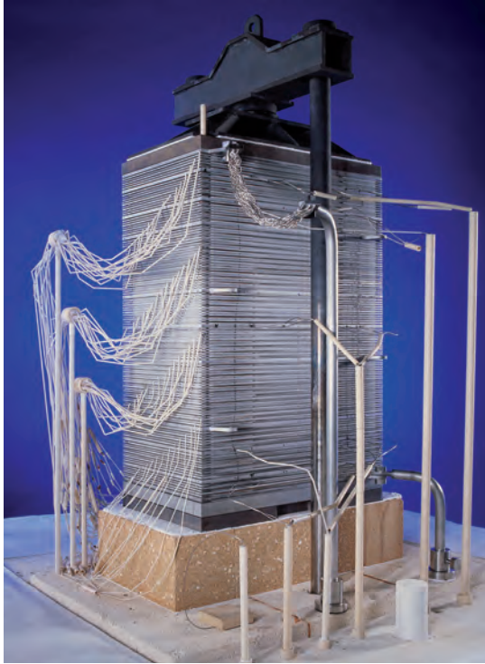
60 cell SOFC stack manufactured and tested at Forschungszentrum Jülich, Germany. The stack delivers around 13 kW of electrical power
